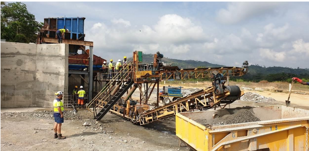
Figure 3: Kimberlite Waste Sorting Belt
