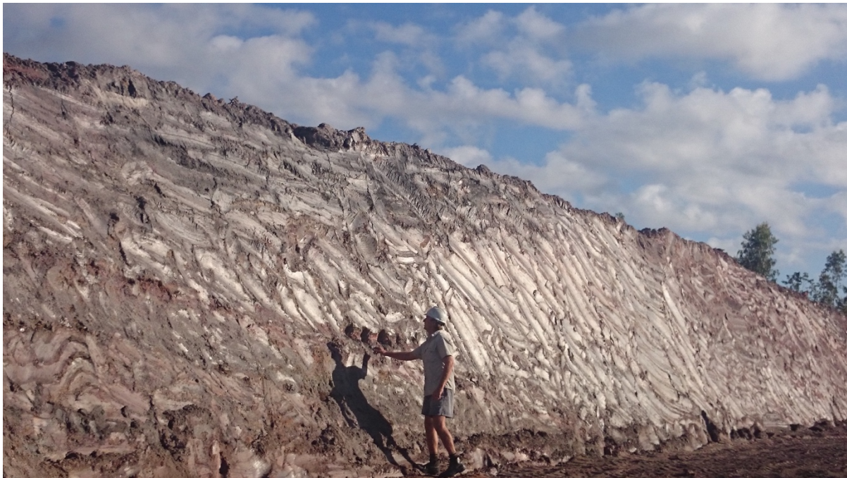
Figure 3: Mining of soft, weathered, graphite rich regolith at the Graphmada Mine.
