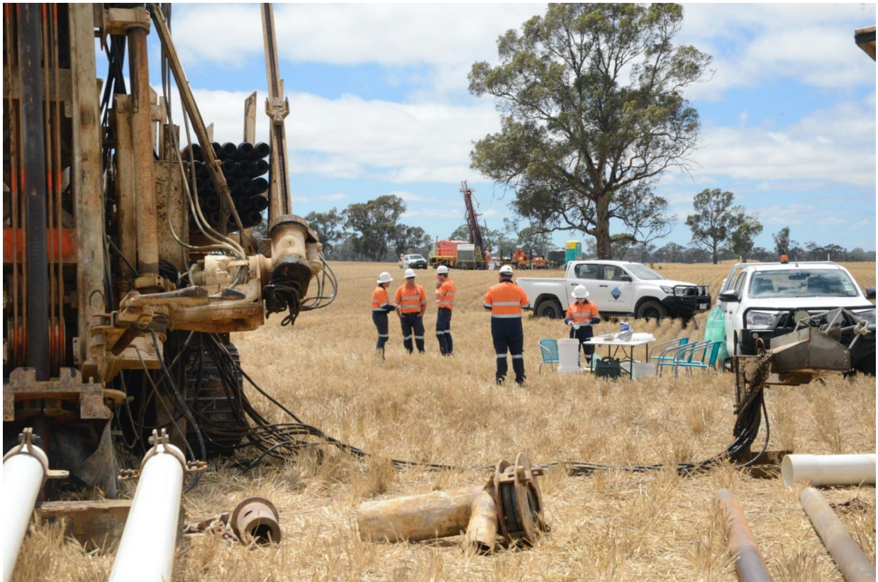
Fig5. RC rig in the foreground, NSM field team preparing to sample RC samples and diamond drilling rig in the background. January 2021
