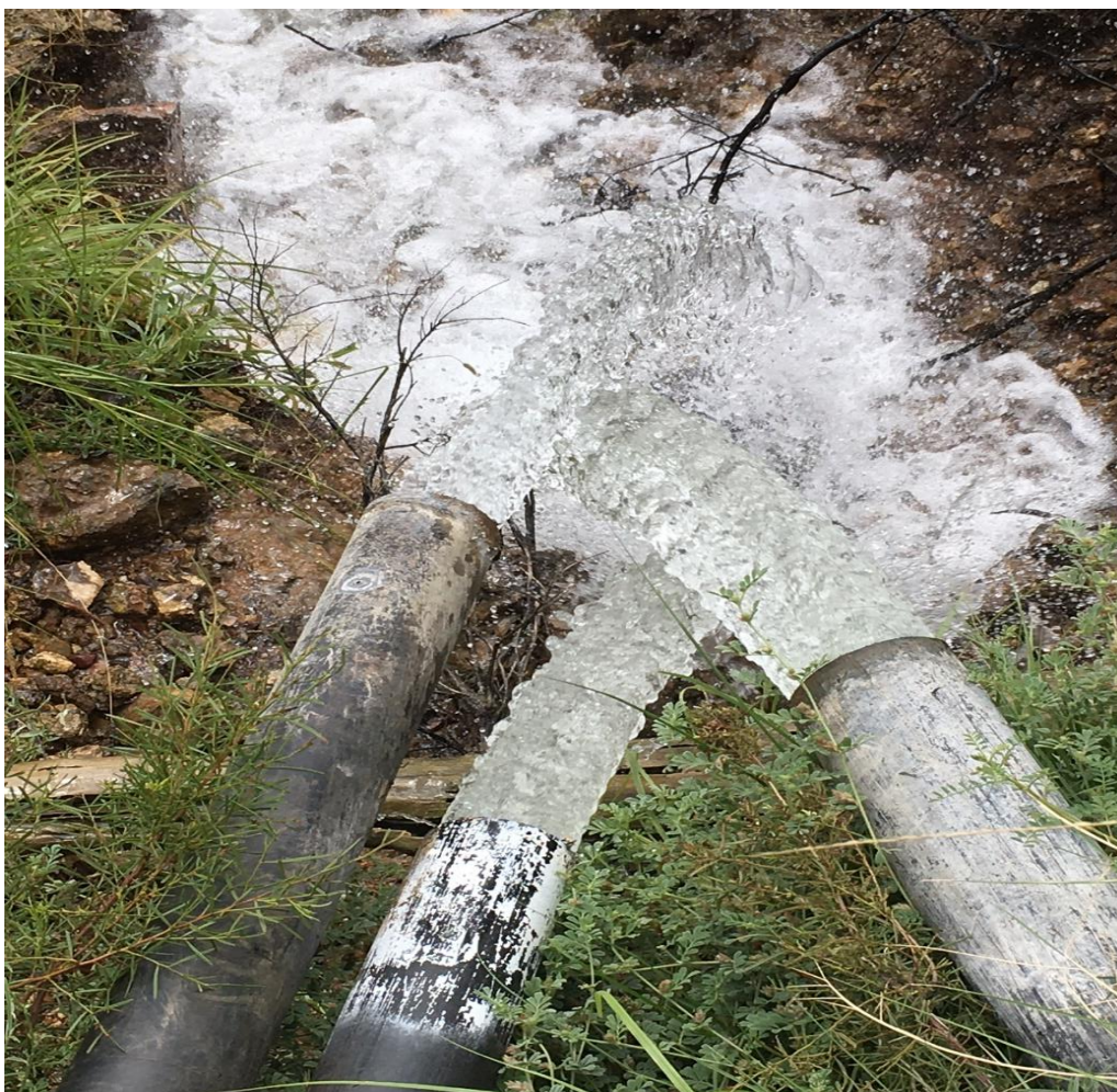
Figure 13: Dewatering bores into evaporation ponds at Mt Freda open cut to 200m.
