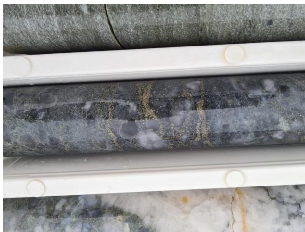
Image 2: Well developed conglomerate zones with visible Pyrite mineralization from hole RLKPDRE-22
