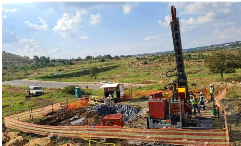
Image 1: Diamond drill team in operation at the WBP.
