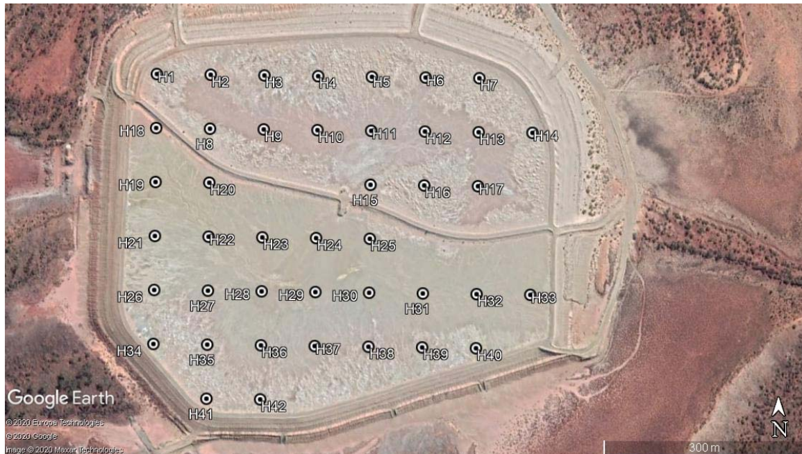
Figure 8 – Planned drill hole location and pattern of HanTails TSF
