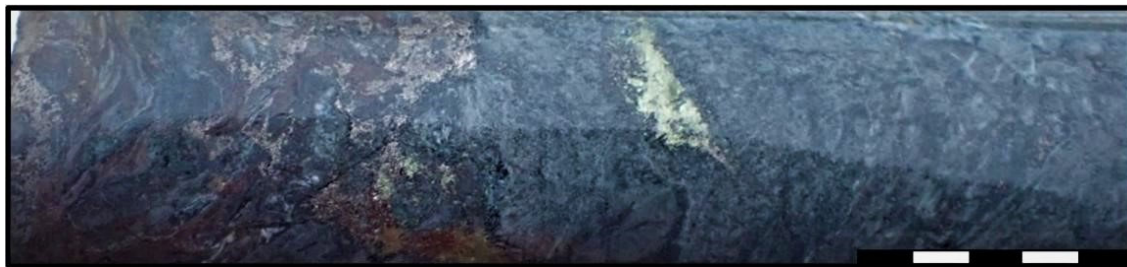
Picture 2: Drill core from KIODD002 (92.7m) – blebs of pyrrhotite-sphalerite-chalcopryrite hosted in quartz-chlorite-actinolite altered volcanic siltstone
