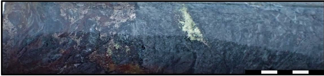
Picture 2: Drill core from KIODD002 (92.7m) – blebs of pyrrhotite-sphalerite-chalcOPYrite hosted in quartz-chlorite-actinolite altered volcanic siltstone
