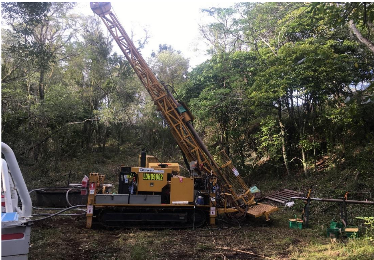
Photo 2: Diamond Drill Rig at the Amamoor South-Central Manganese Prospect
