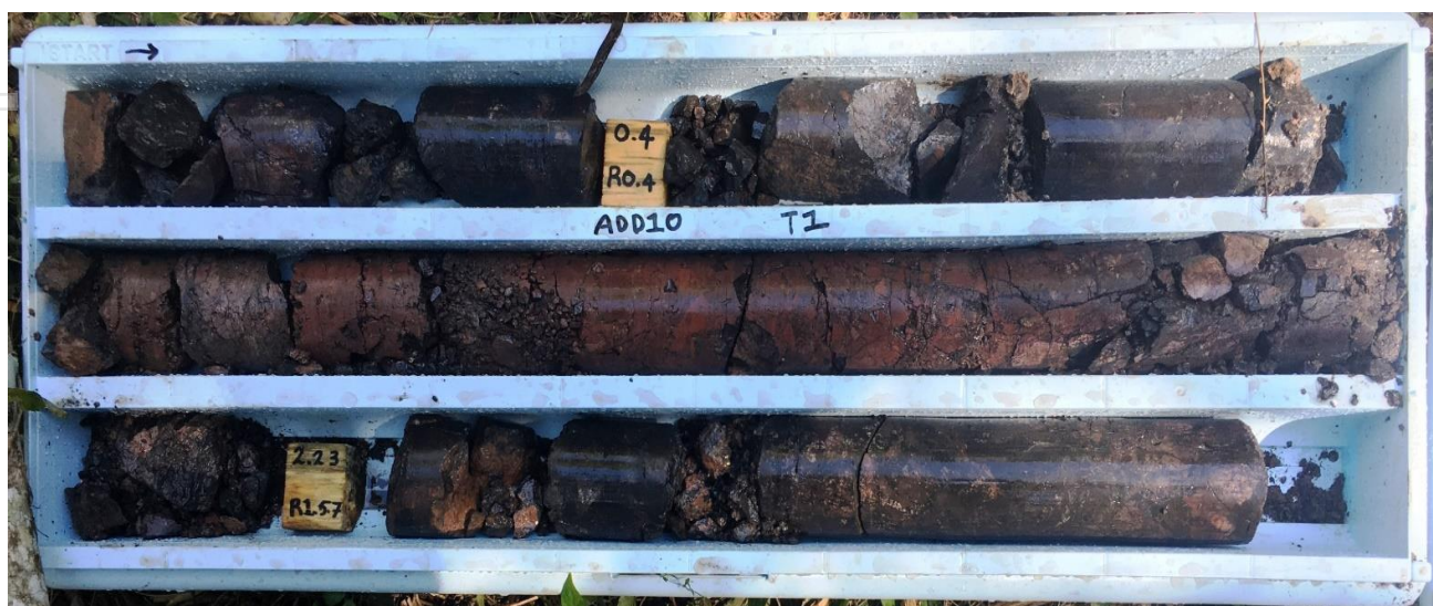
Photo 1: Amamoor Northern Zone Hole ADD010 – 0 to 2.74m, strongly fractured black manganese with minor silicified jasper fragments
