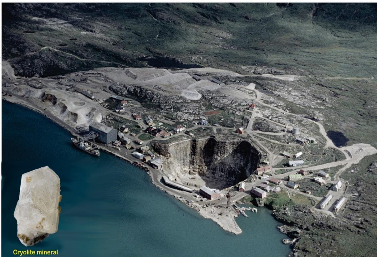
Photo 4: Aerial image of Ivittuut and the cryolite mine in 1960, showing the working open-pit, mine infrastructure, ore and waste dumps and ship loading facilities.
