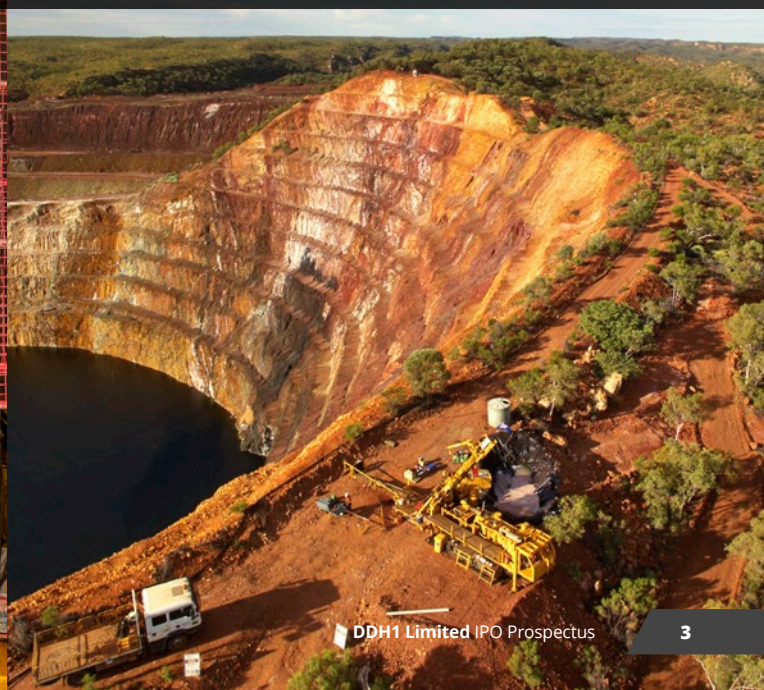
DDH1-Rig 29: Tracked UDR650 Multipurpose Core Rig, North Queensland
