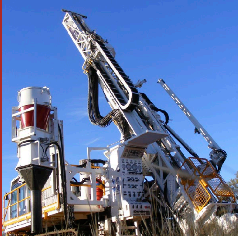
Strike Drilling-Rig 4: Austex X350 dual purpose Aircore/RC Tack mounted rig Midwest WA
