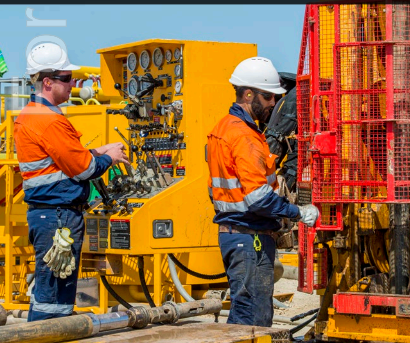
DDH1-Rig 16: Evolution 3000 Multipurpose Core Rig, South West WA
