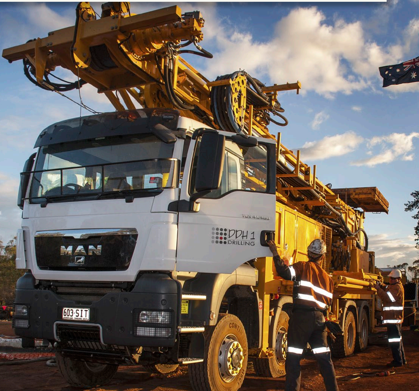
DDH1-Rig 17: Evolution 3000 Multipurpose Core Rig on MAN 8WD truck
