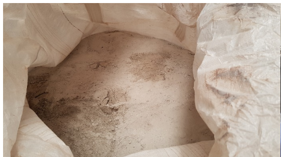
Figure 1. Initial sample of spodumene-bearing drill chips for testing.
