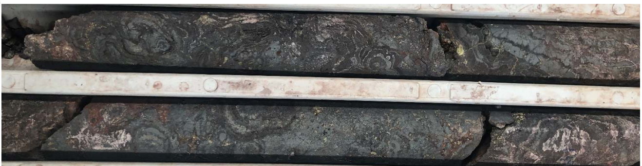
Figure 3: VUD018, colloform massive hematite breccia at ~1387m, NQ core.
