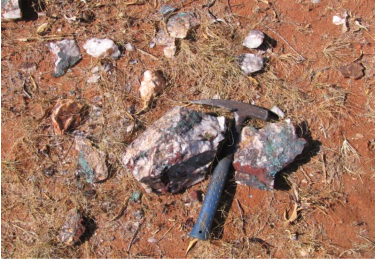
Figure 13. Gossanous veins with green malachite staining at Bruce's Gold Prospect; samples yielded 1.9g/t gold and 1.6% copper 1 .
