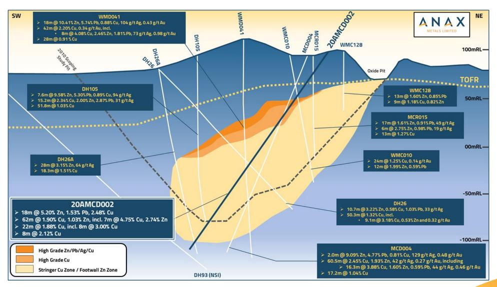
Mons Cupri Oblique Section showing 20AMCD002 and select previous drill holes. Note: A number of holes have been omitted from the section for ease of display; only the most significant intervals are displayed - Refer to ANX ASX Announcement 25/11/2020
