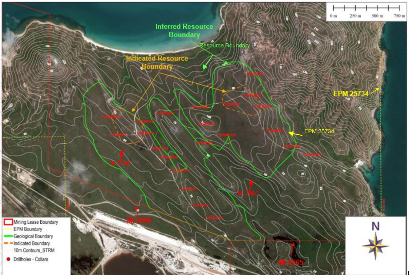
Figure 1. CFS Project - Eastern Resource Area - Surface Dune Boundary (green line)
