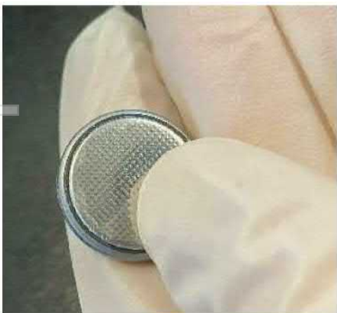
Figure 1: Novonix – Freshly assembled lithium-ion battery coin half-cell with Lake's lithium product
