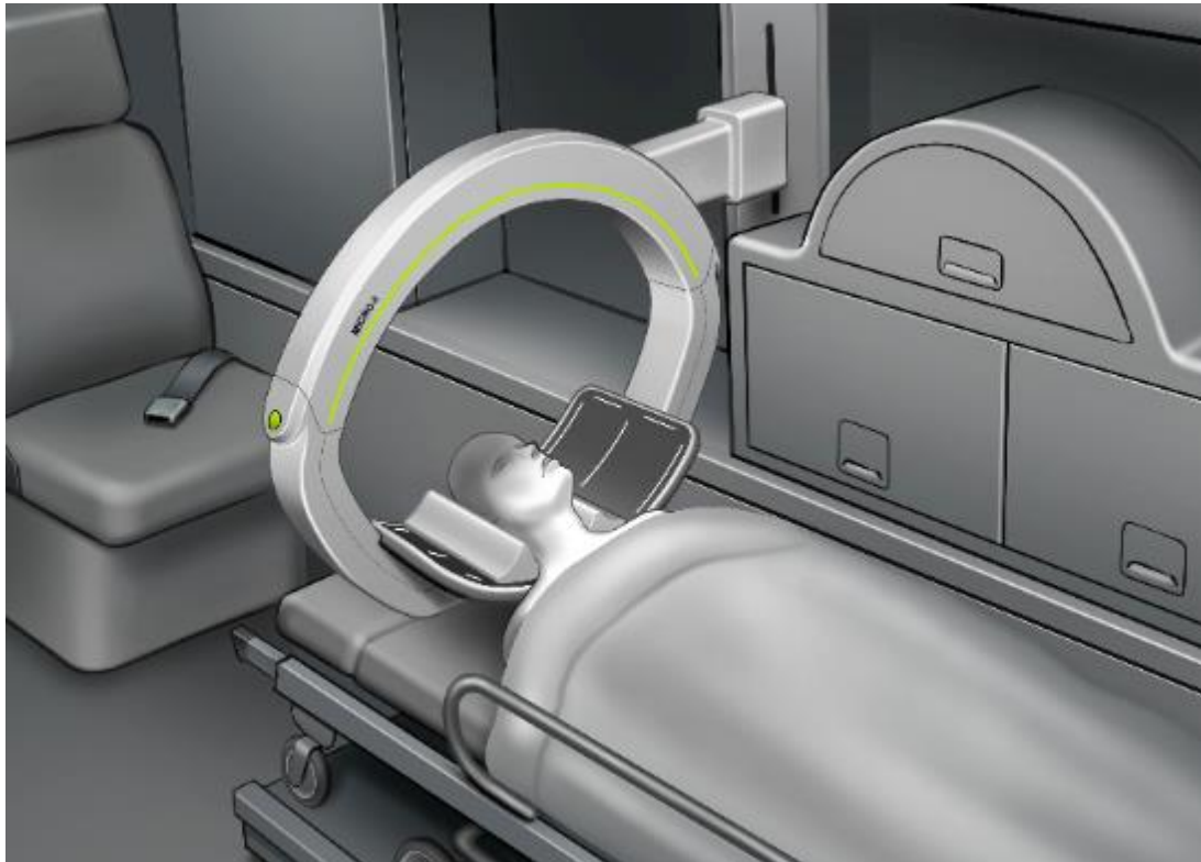
Illustration of Micro-X's concept design for a stroke imaging Brain CT fitted in an ambulance
