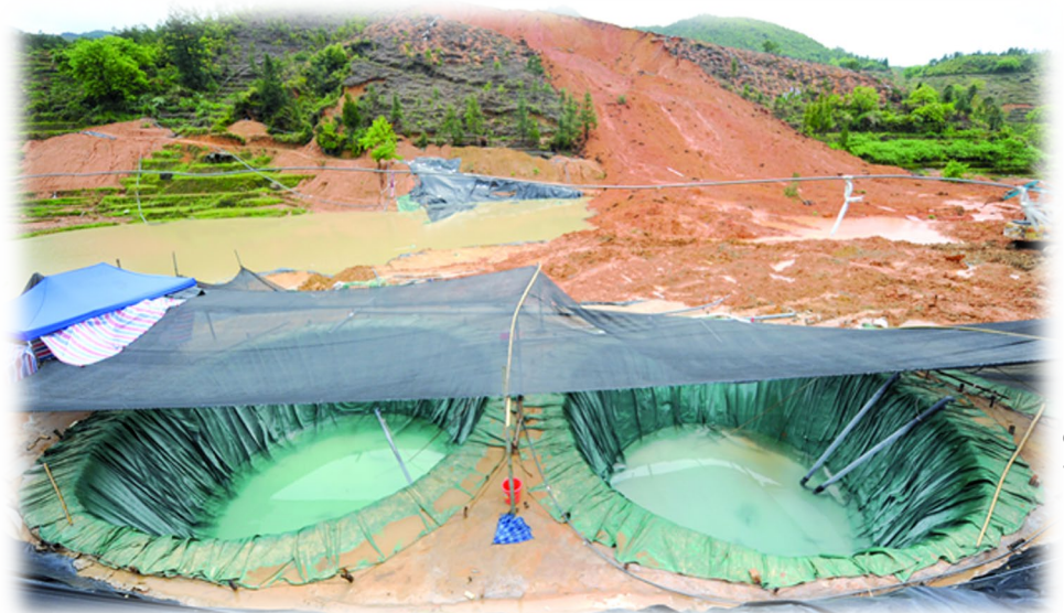
Southern China in situ leach mining operation
