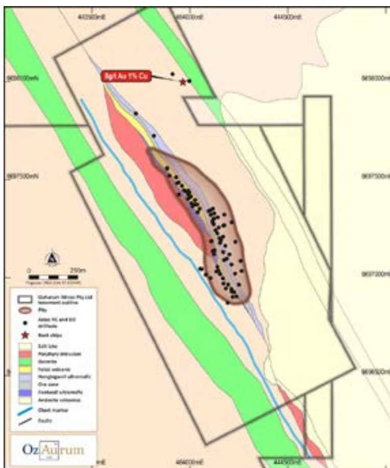
Figure 12: Geological plan of Patricia Mine, after Aztec and NEGE
