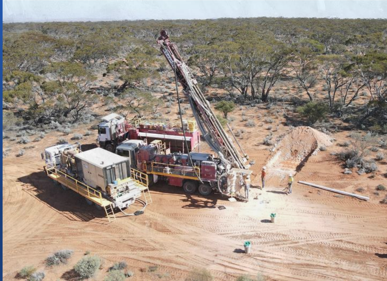
RC rig drilling at Paris
