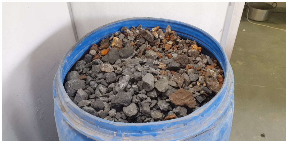
Primary crush product 12mm + via Jaw crusher
