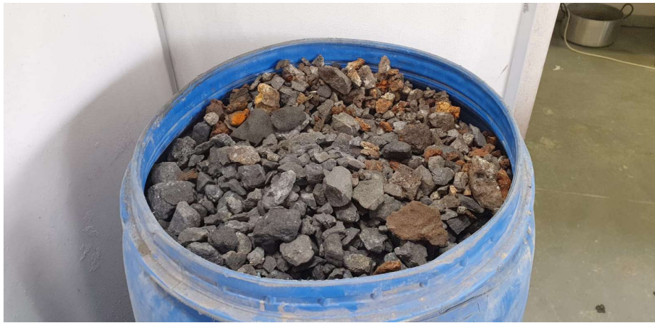
Primary crush product 12mm + via Jaw crusher
