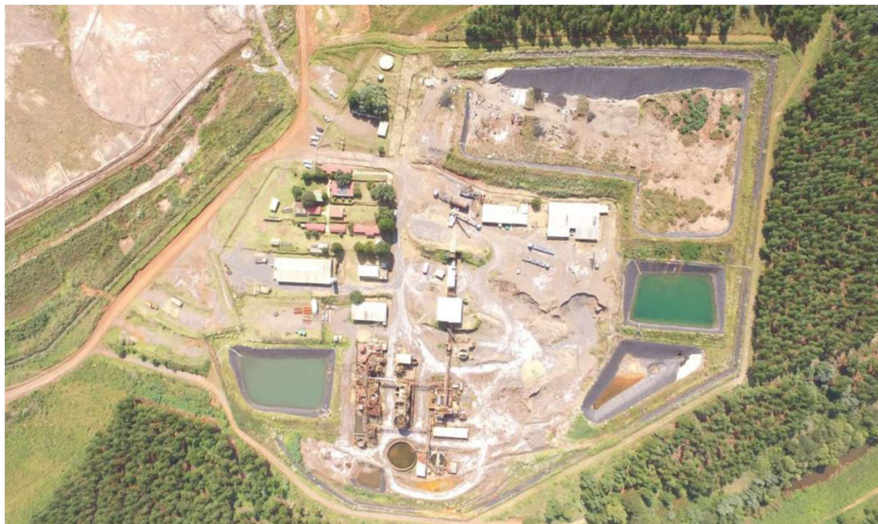
TGME GOLD PLANT FOOTPRINT- Tailing Storage Facility (TSF), admin building, machinery shed, water, and Power onsite
