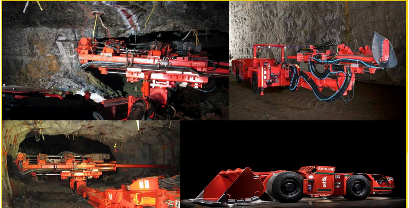
Sandvik low Profile LHD – At a height 1.6 m designed for operation in narrow-reef drill drives
