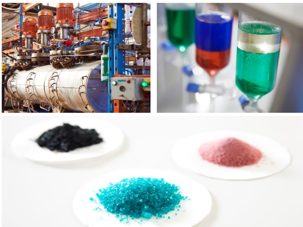
Figure 5: Collage of photographs taken of Australian Mines' demonstration scale processing plant in Western Australia, including images of the final cobalt sulphate (pink) and nickel sulphate (blue/green) and the intermediate mixed sulphide precipitate (MSP; black), which are routinely being produced.
