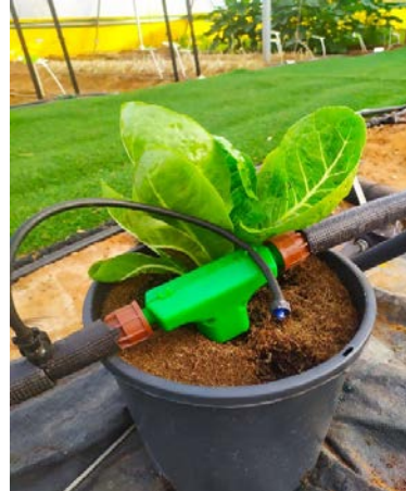
Figures 2 & 3: Heat exchange probe coupled with irrigation and fertigation functionality
