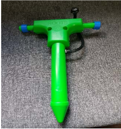
Figures 2 & 3: Heat exchange probe coupled with irrigation and fertigation functionality
