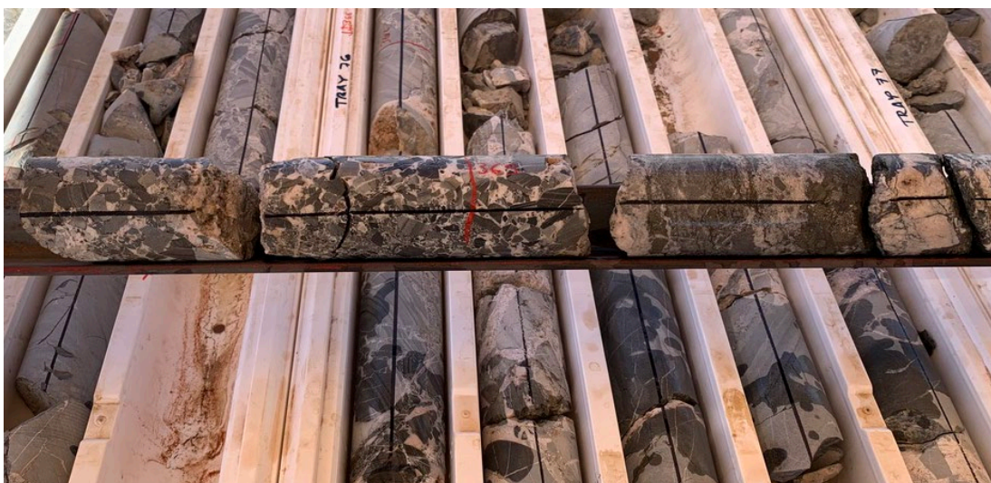
NQ2 core from diamond drillhole 20ALDD0003 showing typical brecciation at approximately 365m downhole.
