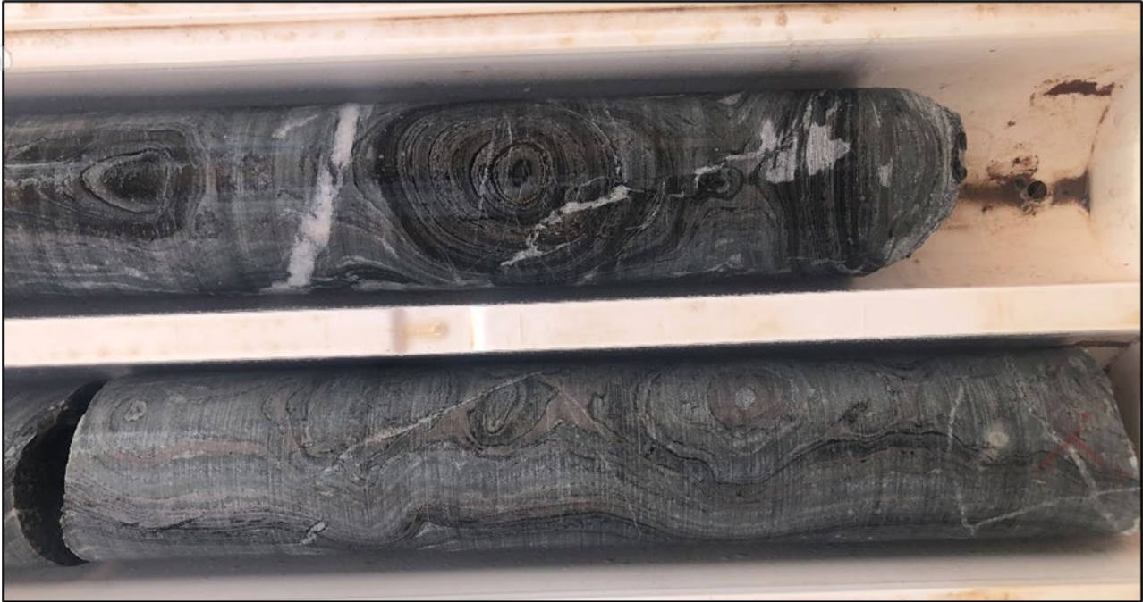
NQ2 core from diamond drillhole 20ALD0006 showing basin and dome interference patterns in tightly folded quartz sandstones (145m – 146m downhole depth).
