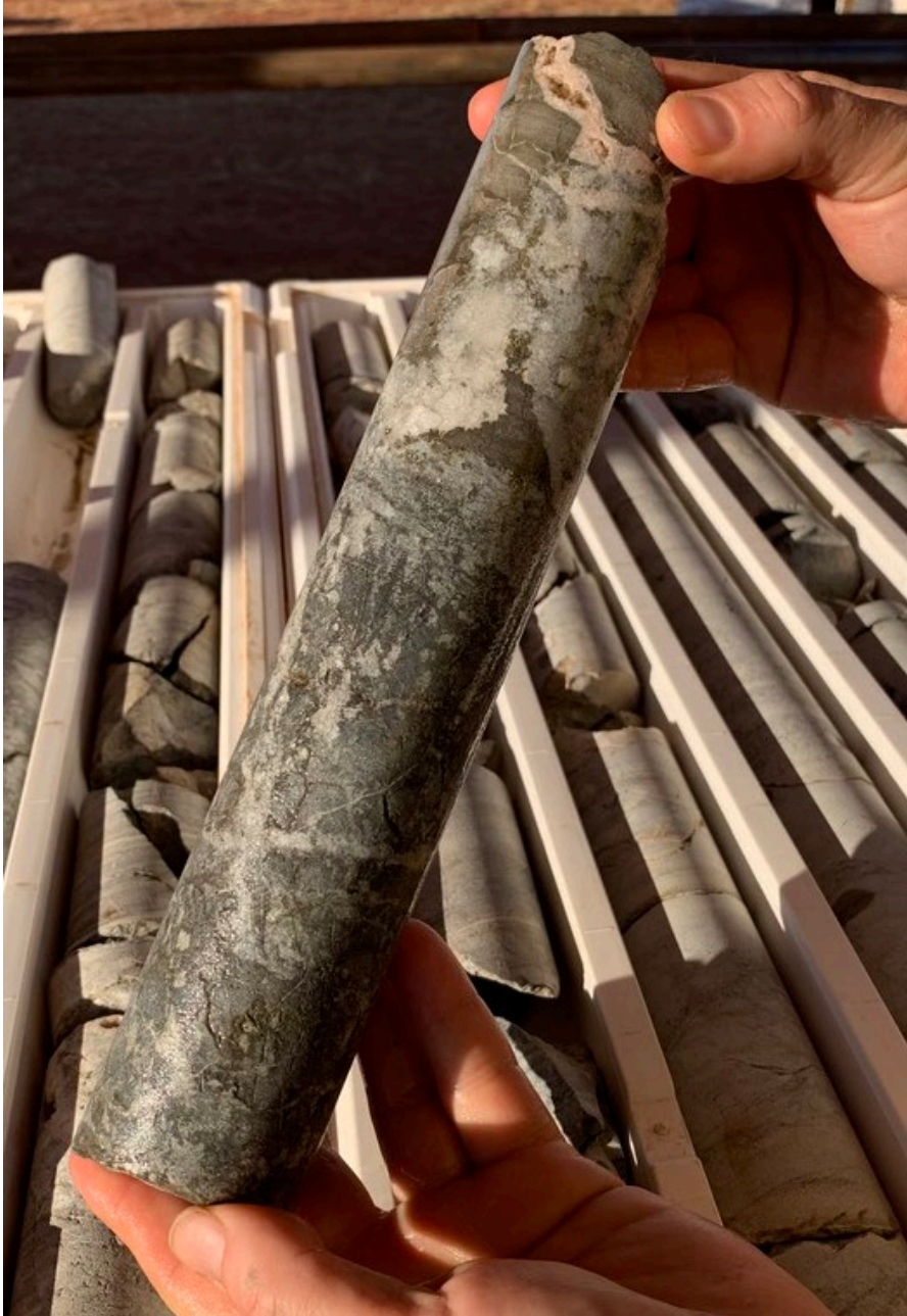
NQ2 core from diamond drillhole 20ALDD0003 showing pyritic quartz-carbonate veining at approximately 500m downhole.
