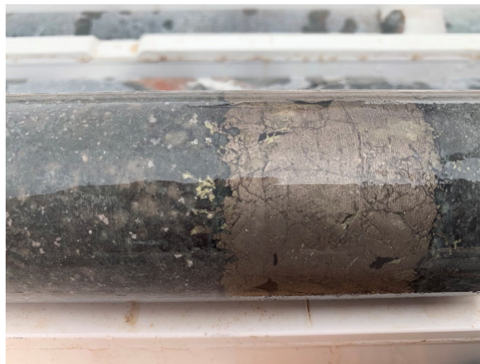
NQ2 core from diamond drillhole 20ALDD0007 showing dolerite hosted massive pyrrhotite (approx. 5cm) with fine chalcopyrite at approximately 119m downhole.
