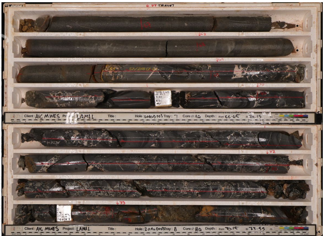
NQ2* core from diamond drillhole 20ALDD0003 showing intense quartz-carbonate stockwork veining immediately below the cover-basement unconformity at 68.7m downhole.
