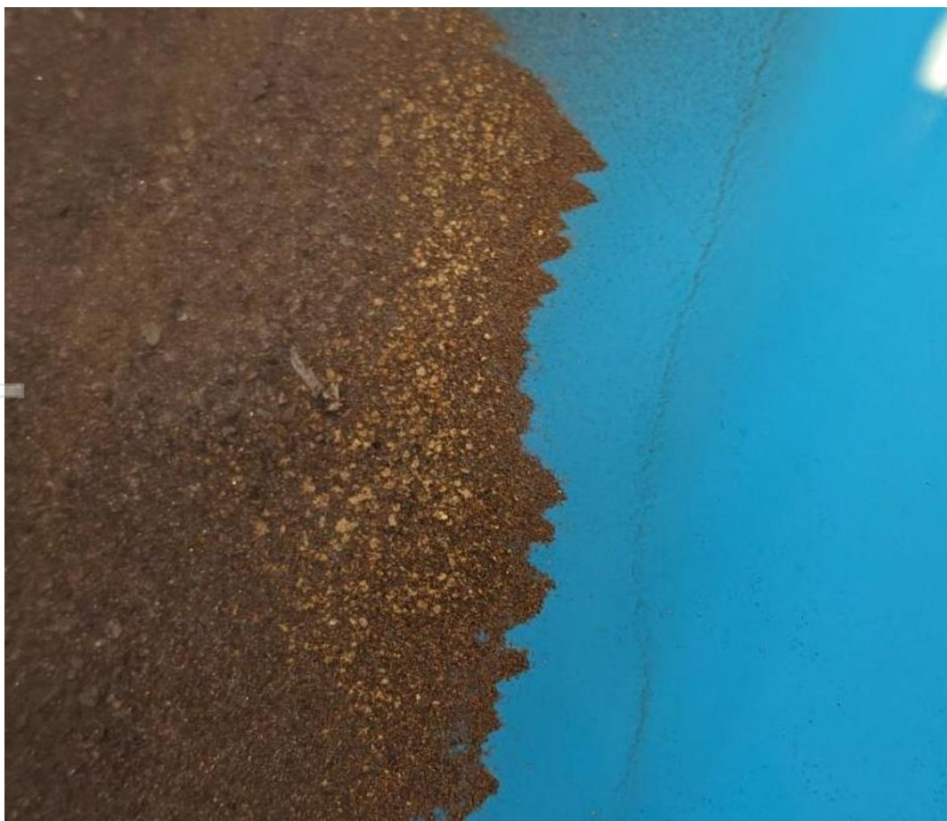
Figure 4 Free gold in Knelson gravity gold concentrate
