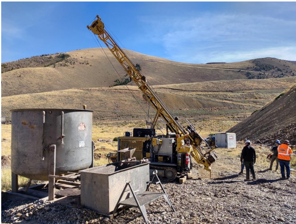
Figure 2: Diamond rig setting up on the drill pad for hole ZBF003 at South Sammy
