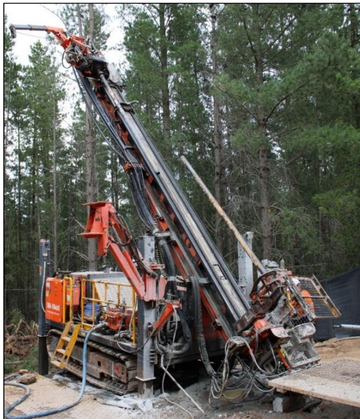
Figure 5: Diamond drill rig in operation at the Lightning Prospect, Castlemaine Gold Project (EL006679)
