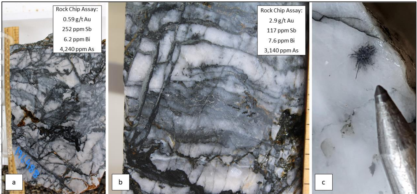
Figure 8: Rock samples collected from the Fentiman's South historic mine waste dump (scale ruler in cm): (a) mineralised quartz vein with abundant stylonite and breccia textures; (b) disseminated sulphides (arsenopyrite, stibnite and pyrite) within a stylonitic and brecciated quartz vein; and (c) coarse stibnite ( \text{Sb}_2\text{S}_3 ) crystals and thin stylonites within a mineralised quartz vein
