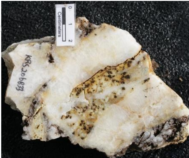
Figure 11 – Outcrop from Geum Mar, KRS206833. Comb-cockade banded quartz vein with disseminated sulfides, 3.88g/t gold, 2.4g/t silver.
