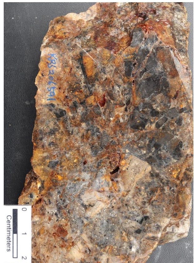
Figure 9 – Float at Thistle Zone, KRS206591. Rhyolitic tuff and volcanogenic carbonaceous mudstone breccia with FeOx stain. 4.49g/t gold, 635g/t silver.
