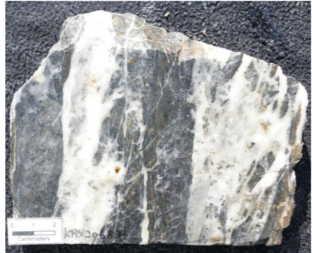
Figure 12 – Float at Geum Mar, KRS206834. Sheeted network quartz vein breccia hosted in siltstone/shale with iron/sulphide oxides. 24.0g/t gold, 11.5g/t silver.
