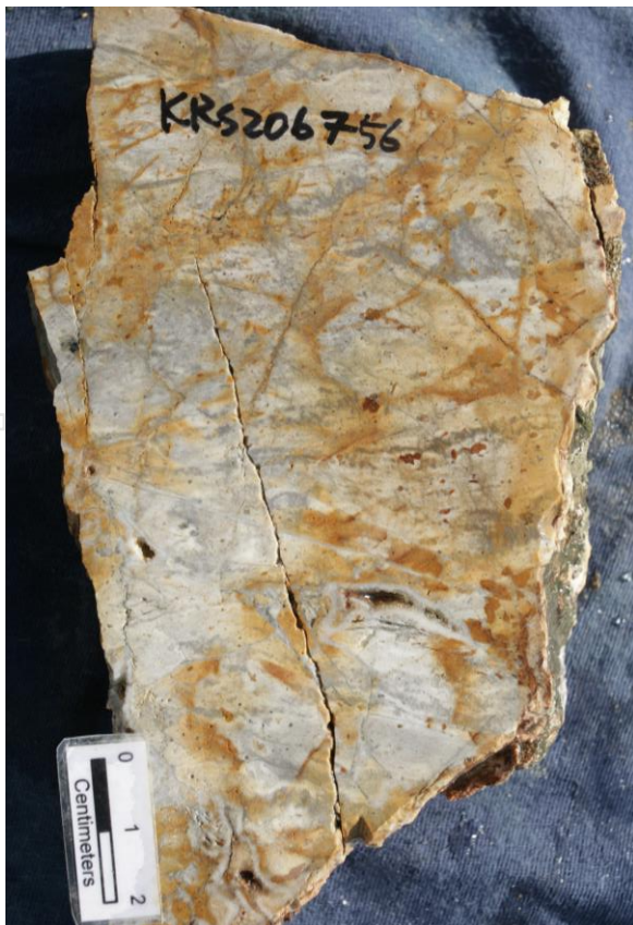
Figure 8 – Outcrop from Nettle Zone, KRS206756. Silicified rhyolite with sheeted-bladed-microcrystalline-comb quartz and hydraulically brecciated veining. 1.54g/t gold, 35.2g/t silver.
