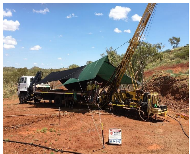
Photo 2. Diamond Core rig currently infill drilling at Comstock, 300m West of Falcon Golden Mile.
