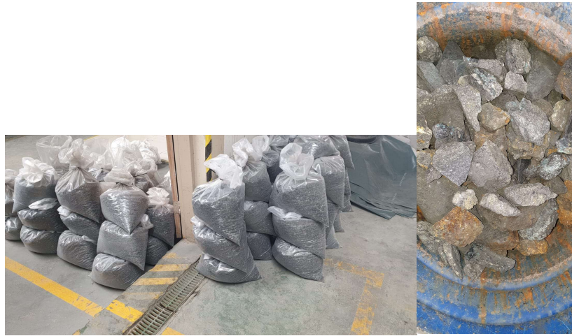
Underground ore samples from mine face 20+ mm sample size (5 tons of sample collected from underground mine)
