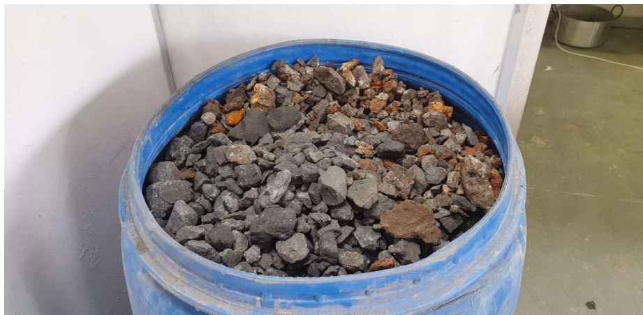
Primary crush product 12mm + via Jaw crusher
