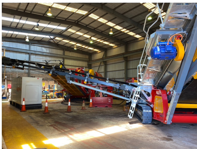
Figure 2: Crusher and dry screen undergoing final tests before mobilisation.
