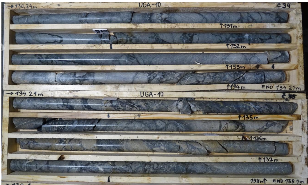
Figure 4: UGA-10 drill core; interval from 130.9m to 138.1m (down-hole) showing quartz filled vein/stockwork/breccia structures, variably rich in fine to very fine grained sulphides (mainly pyrite/marcasite) and hosted within strongly argillic altered andesite host rock. Traces of visible gold identified at 135-135.1m.
