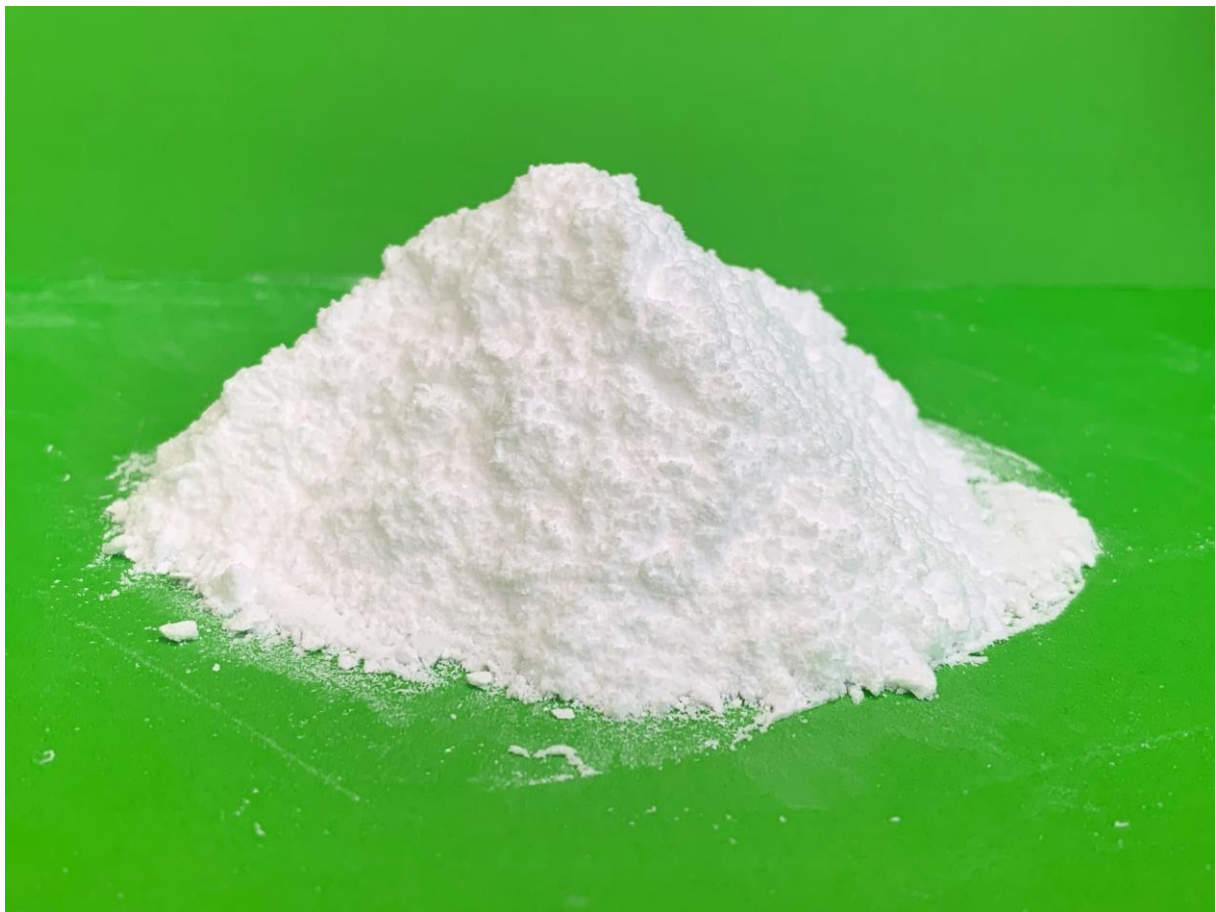
Figure 1: Primary Lithium Sulphate produced under metallurgical testing for AVZ's planned Manono Lithium Sulphate Plant
