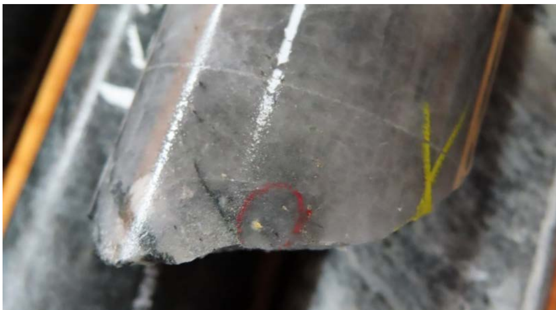
Figure 5: Visible gold grain in quartz-tourmaline vein, hole EM20-132, ~532.7m (core diameter 47.6mm)
