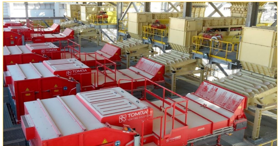
Nameplate capacity is the 1800 tons per hour XRT-based sorting plant at the Umm Wu'al phosphate mine in Saudi Arabia
