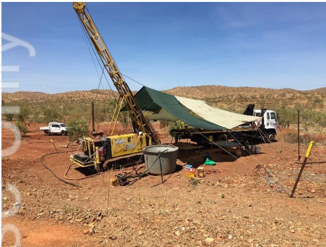
Photo 1. Diamond core drilling at Comstock.
