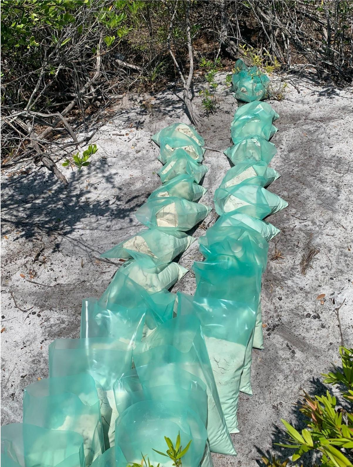
**Figure 3: Sample bags with white sand collected from one drill hole during the December 2020 Cape Flattery drill program**
