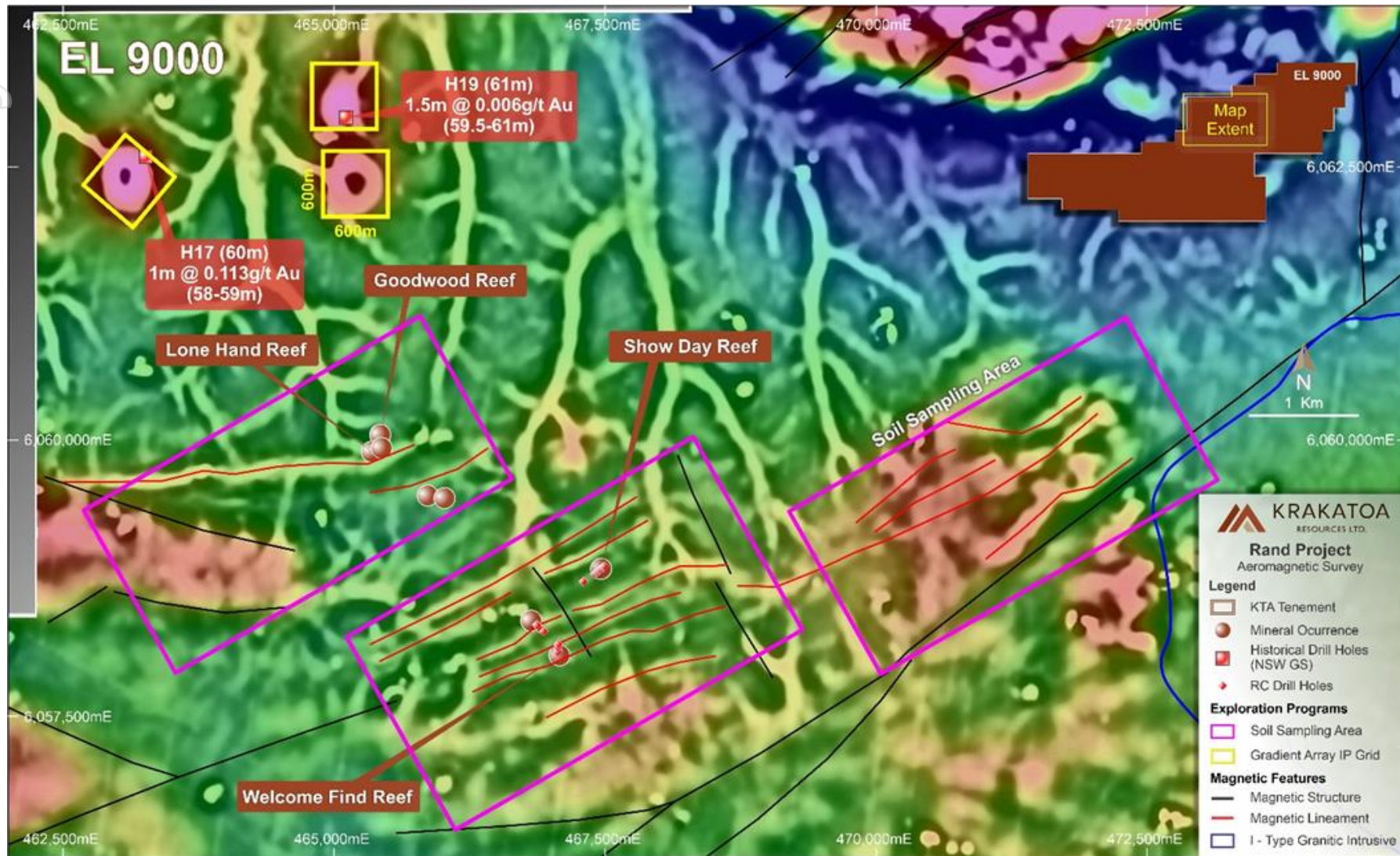
Figure 1 – Priority exploration targets with historical gold workings and GSNSW drilling, on Aeromagnetic TMI-RTP image.
