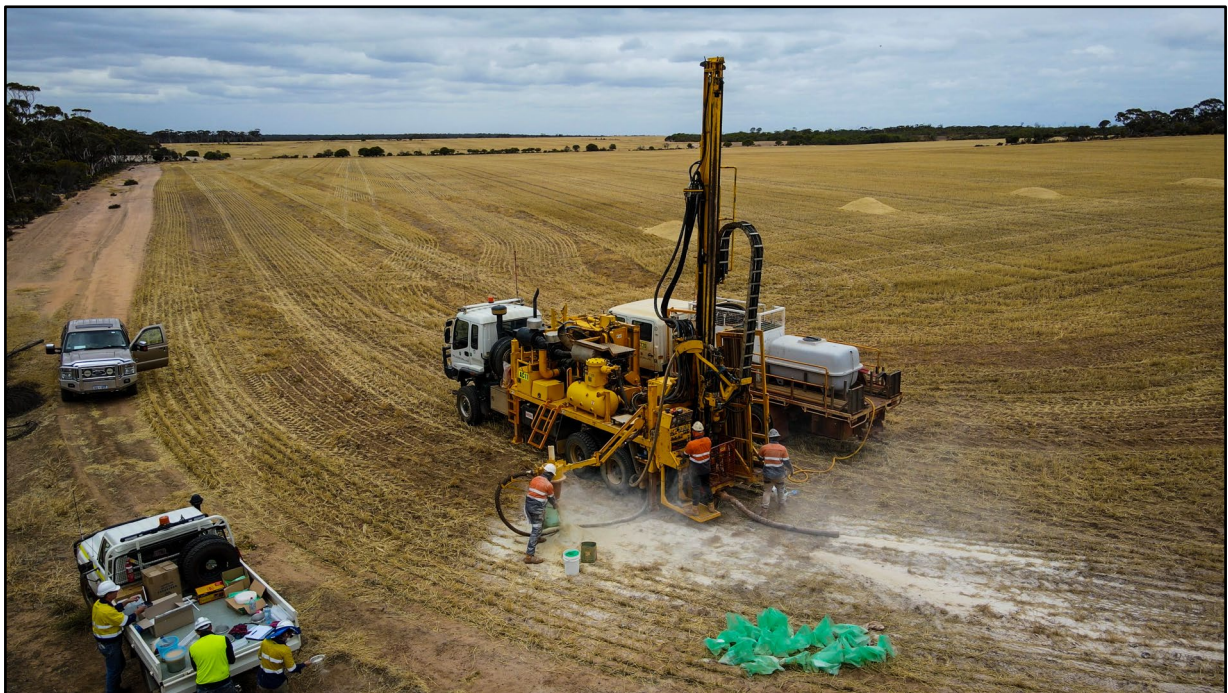
Figure 1: Air-core drilling of kaolinitic clays at the Noombenberry Kaolin-halloysite Project in WA
