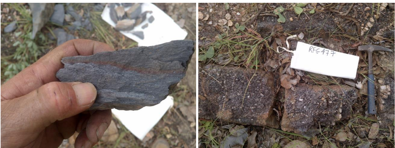
Figure 3. Host rocks for the quartz veins include graphitic schist with notable sulphide alteration (left) and quartz-pebble conglomerate with free gold in intragranular space (right)
