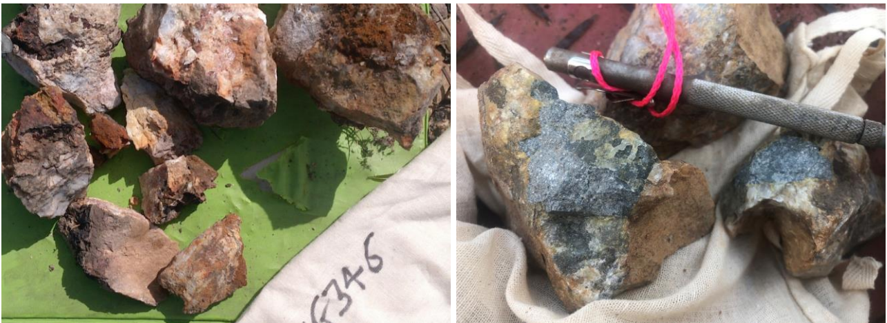
Figure 2. Typical gold-bearing quartz vein from Hurricane Prospect with large vugs of oxide after sulphide (left) and primary arsenopyrite (right)
