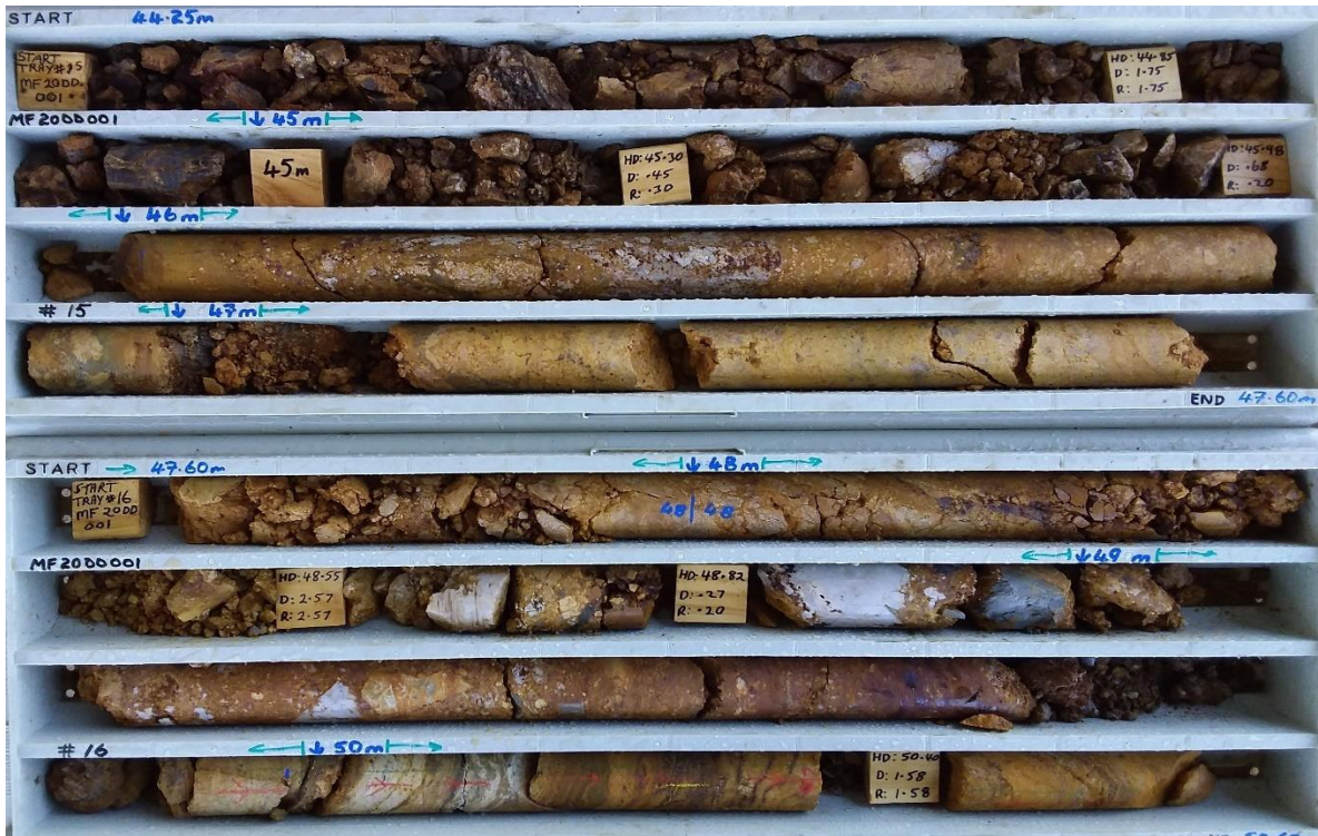
Photo 5. Section of ore zone in MF20DD001: 11m @ 3.6g/t Au from 41-52m incl. 2m @ 13.80g/t Au.
