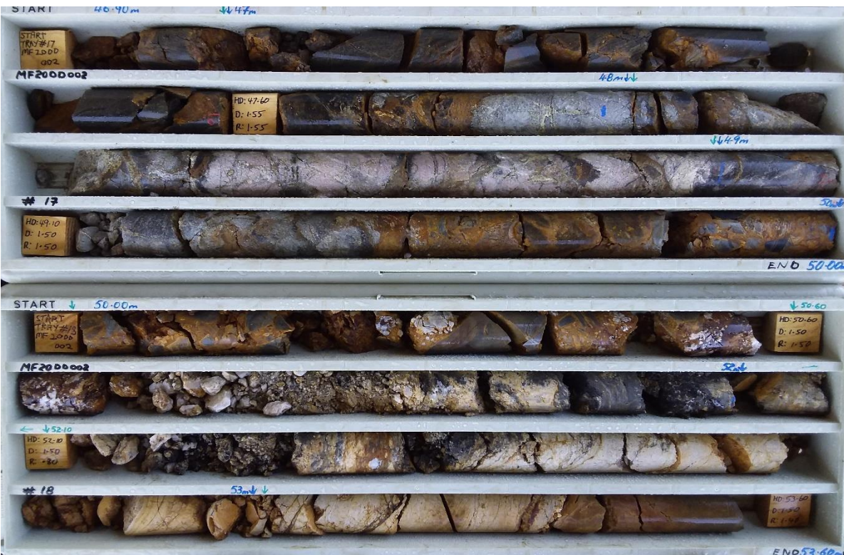
Photo 6. Section of ore zone in MF20DD002: 12m @ 3.54g/t Au from 43-55m incl. 4m @ 8.34g/t Au.
