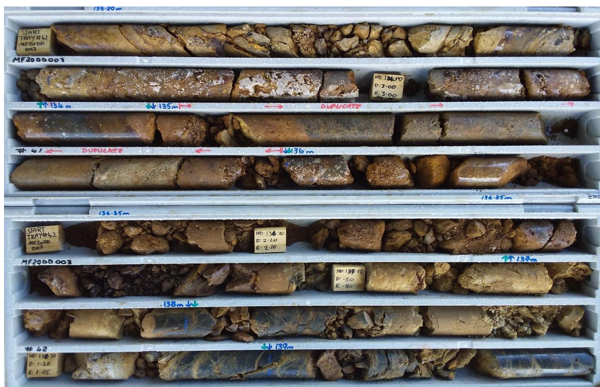
Photo 7. Section of ore zone in MF20DD003: 5 meters @ 11.24g/t Au from 133-138m incl. 3m @ 18.59g/t Au.
