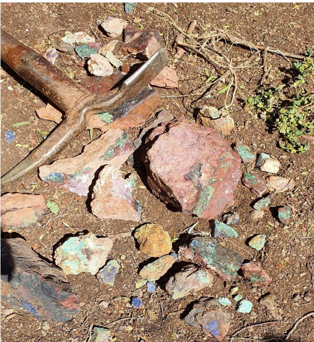
Figure 2: Mine dump samples exhibiting strong copper mineralisation (azurite and malachite).
