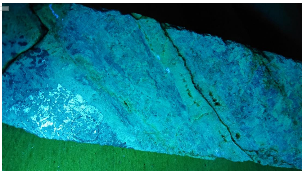
Figure 1 Scheelite in core (CUY007) - (scheelite fluoresces under short wave ultraviolet light)
