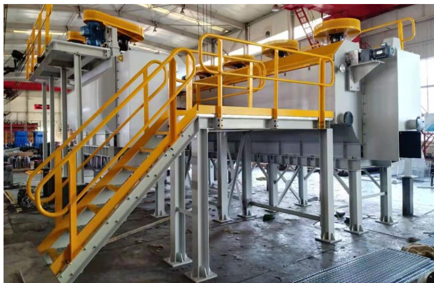
Figure 3: BGRIMM flotation cell model and size for pilot plant
