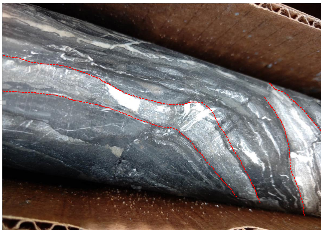
Figure 3: Sulphide mineralisation (highlighted by red) with fold and shear structures developed above intrusive dike in drill hole ZBF001
