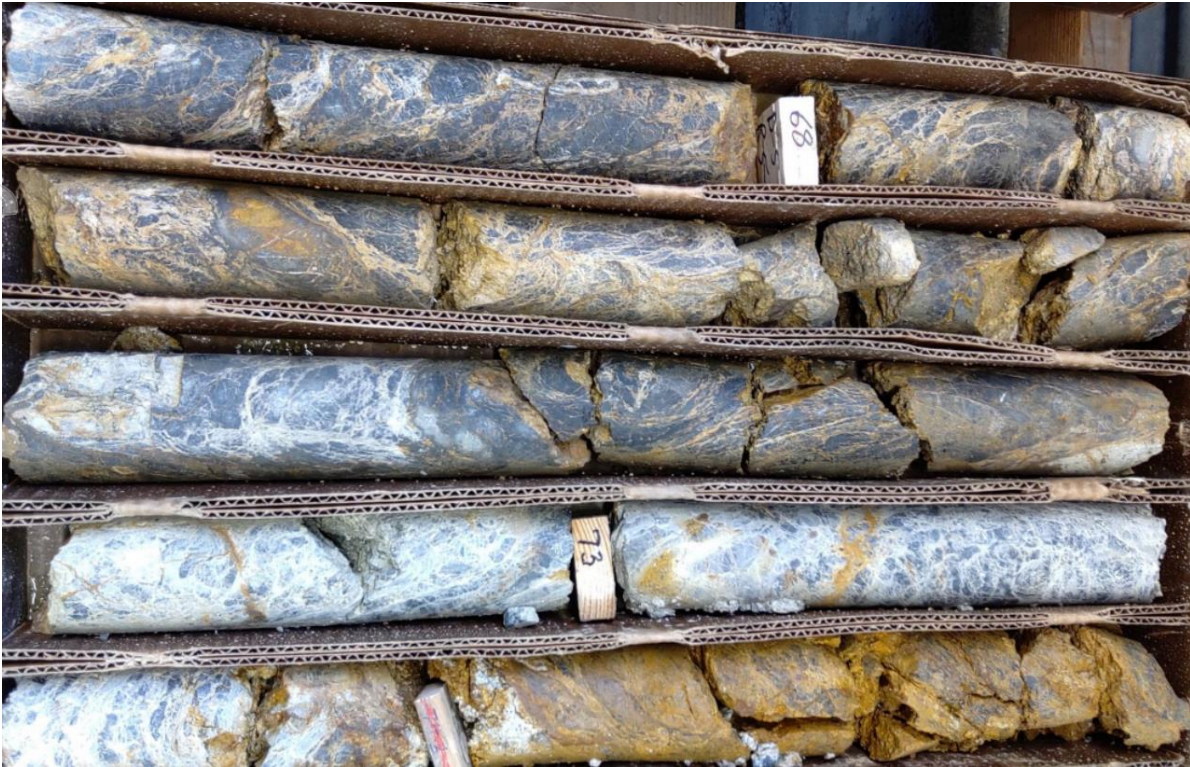
Figure 4: Argillic alteration developed in Unit D intercept with Briens Fault in drill hole ZBF001
