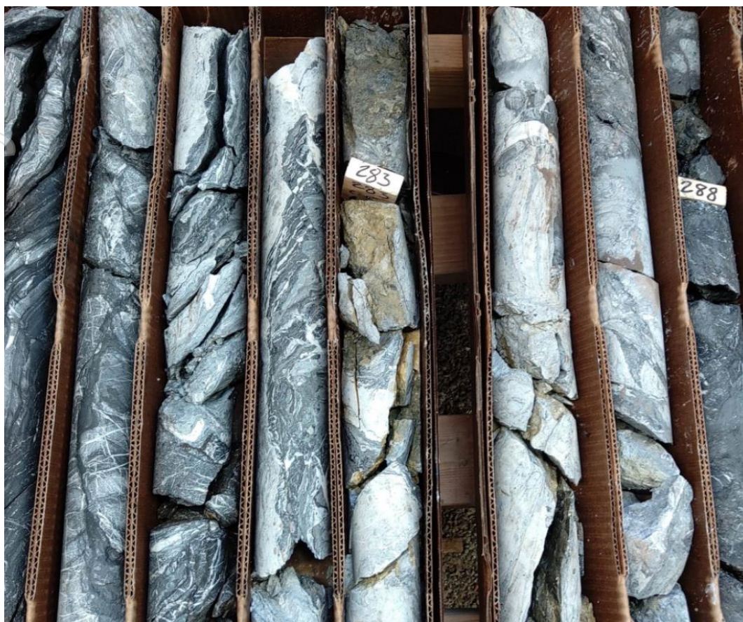
Figure 2: Intermediate to felsic intrusive dikes developed within shear zone in drill hole ZBF001.
