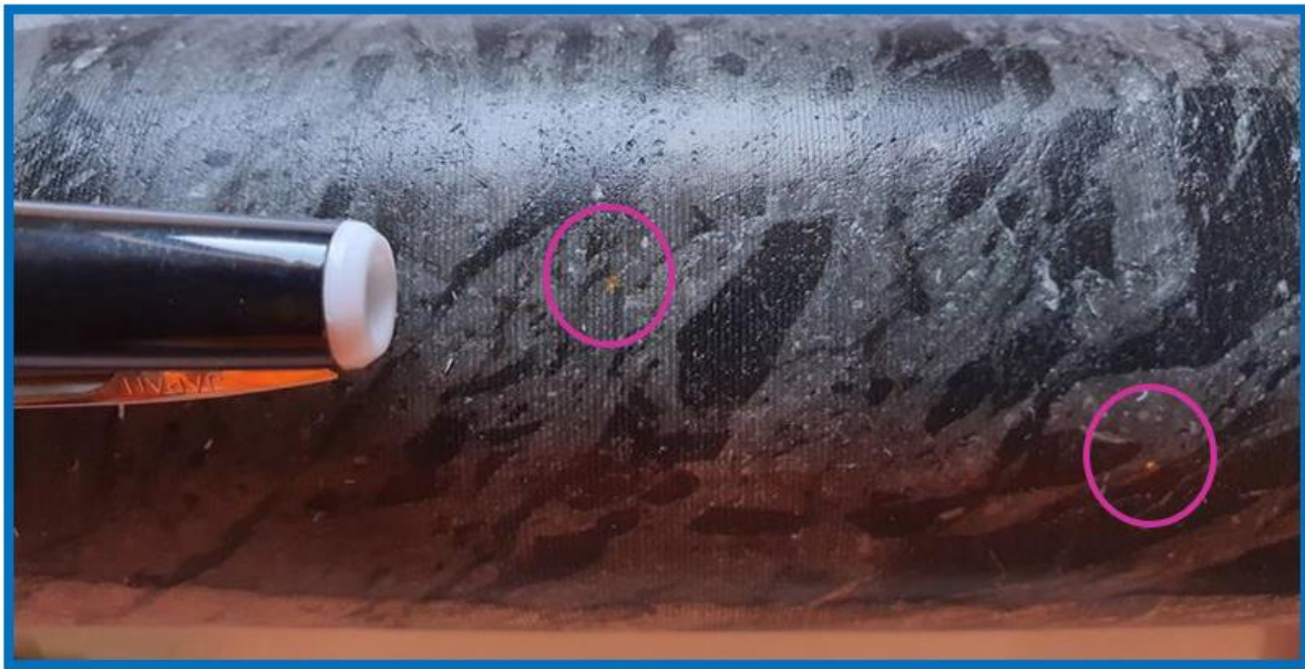
Figure 7: Lionfish HW 357 - visible gold in drillhole ROGC751 (0.28m @ 161.50g/t Au from 37.5m)
