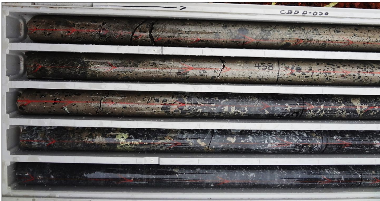
Figure 1. High grade nickel sulphides showing magmatic sulphide textures within the main massive-matrix sulphide zone. The mineralisation comprises breccia rip up clasts within the massive sulphide, interstitial sulphide/crystal intergrowth at the margin, and chalcopyrite segregation within the crystallised host gabbro. Coarse blebs of matrix sulphide are observed between the crystallising host rock (436.7m-441.1m shown).
