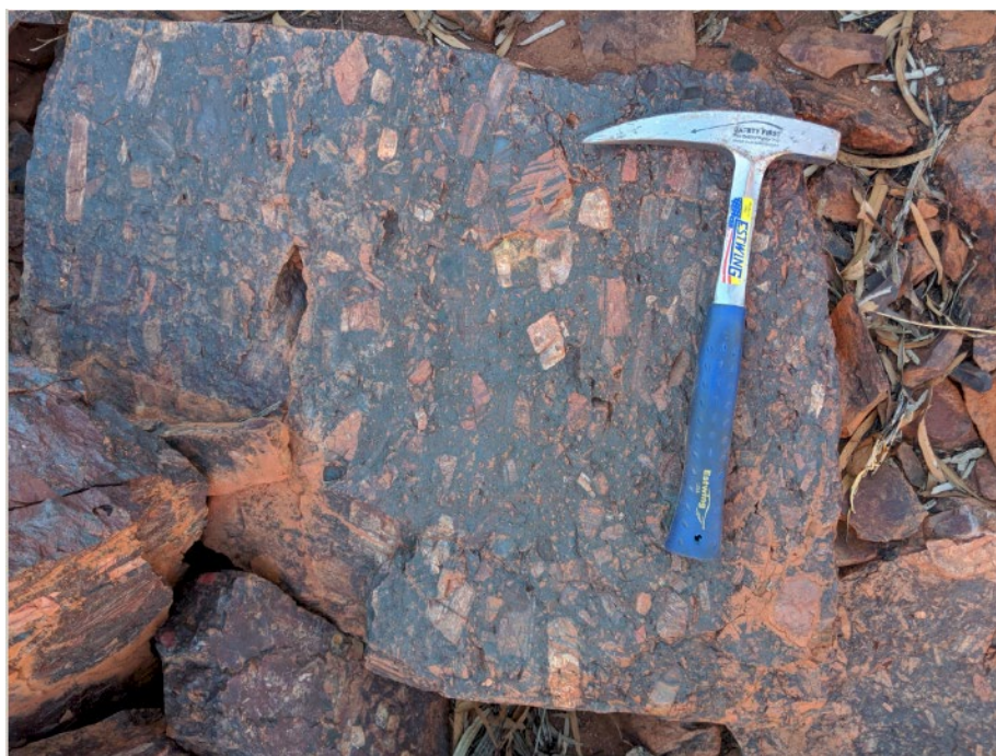
Figure 16: Close up view of “unmineralised” conglomerate with chert and BIF clasts in hematite matrix as found at Paulsens East
