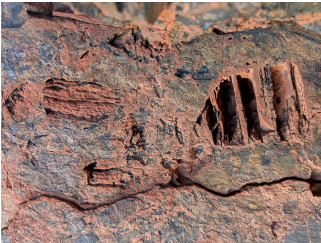
Figure 18: Close up view of "halfway" hematite conglomerate with vughs after chert as found at Paulsens East
