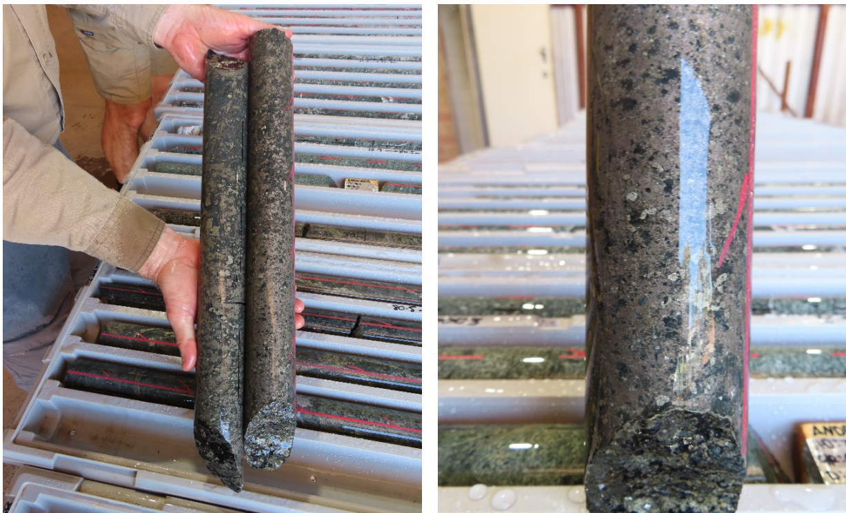
Figure 3: Massive, semi-massive and blebby nickel and copper sulphides in ANDD0003: \sim 79\text{m} downhole
